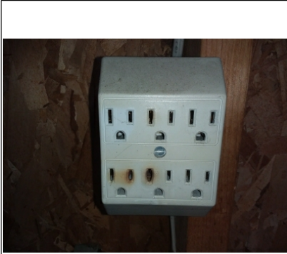
Overheated electrical receptacle
